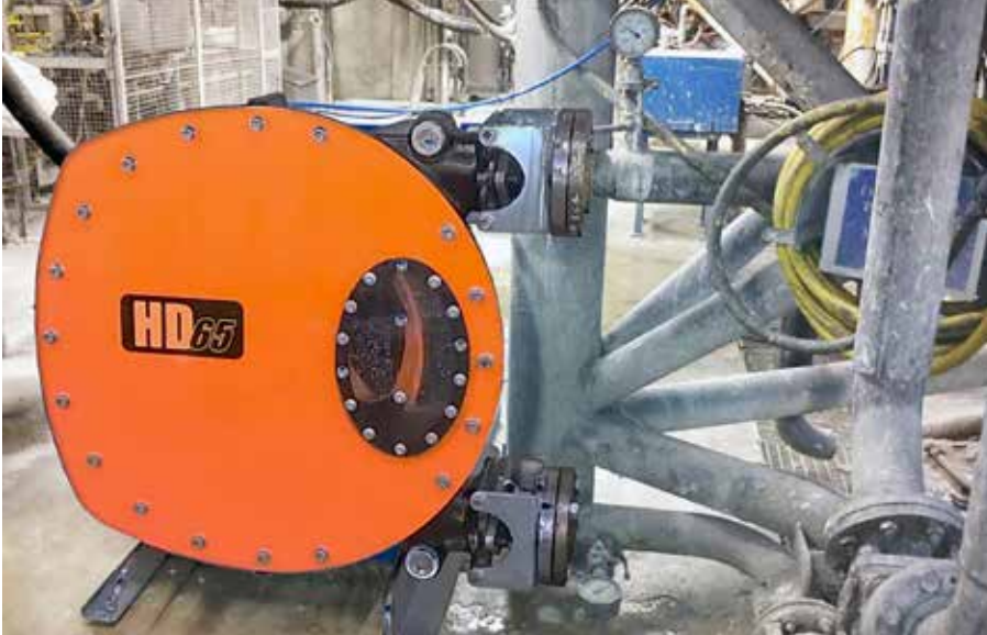
Image 2 (above). Peristaltic (hose) pumps can operate safely, efficiently and reliably in many of the harsh liquid-transfer applications that are prevalent in oil and gas production. Image 3 (right). The peristaltic (hose) pump's ability to maintain volumetric consistency and provide suction lift up to 9 meters (29.5 feet) makes it ideal for 24/7 operating cycles.
