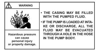
When the hose breaks, there is a risk that the lubricant may be contaminated by the pumped liquid.
