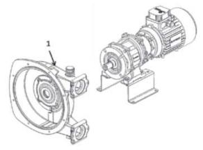
Remove shaft seal 26 from pump body. Put new shaft seal 26 in pump body.
