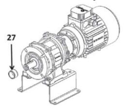
Heat new friction ring at 110 ±10°C / 230 ±50°F.
