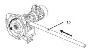
Rotate the pump intermittently until the hose 16 is completely inserted in the body and show equal lengths outside the body on both ports:
