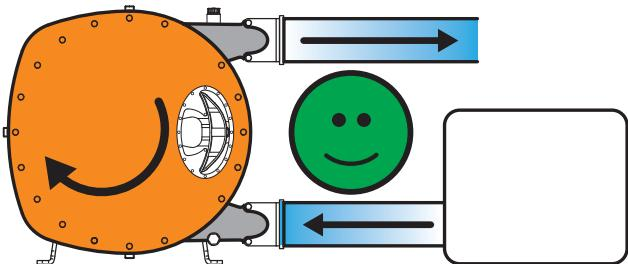
**EN** **Caution / If the fluid is loaded, with the risk of sedimentation, SUCTION from above is imperative.**
