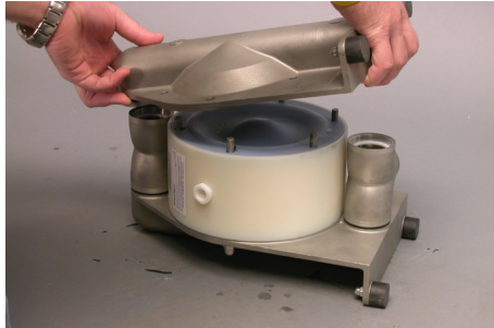
Remove side housing [1] and suction/discharge ports [2].
