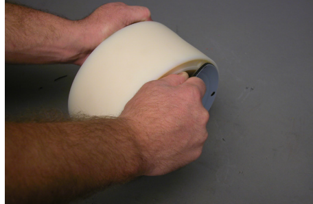
Screw one diaphragm [14] counter clockwise off the shaft [13].
