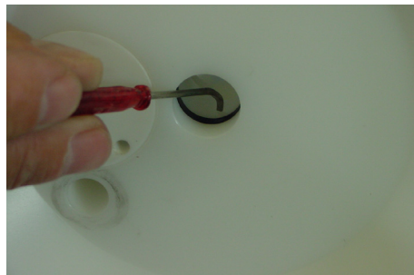
Remove both parts of the shaft piston rings [17] from their grooves carefully (do not damage the edges in the center block; a re-assembly of the same piston rings is impossible; they have to be replaced). Unscrew the muffler [20], the air inlet [18] and the air filter [19] out of the center block [16].
