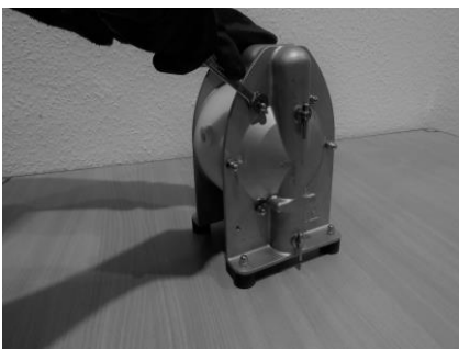
Loosen nuts of the housing bolts (19) on one side of the pump.
