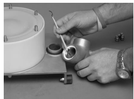
Draw the O-rings port outside [10] off the side housings [1]. Remove the inner O-rings [9] out of the ports [8].
