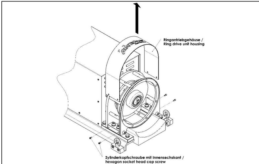
Lose the hexagon socket screw and disassemble the ring-drive-unit-housing up to the top.
