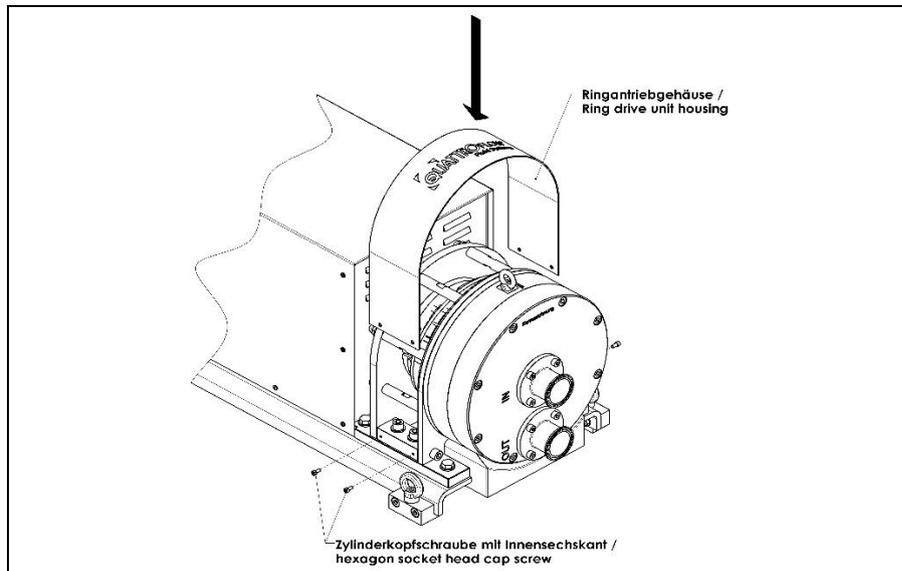
Assemble the ring-drive-unit-housing and fasten it by screwing in the hexagon socket screws.
