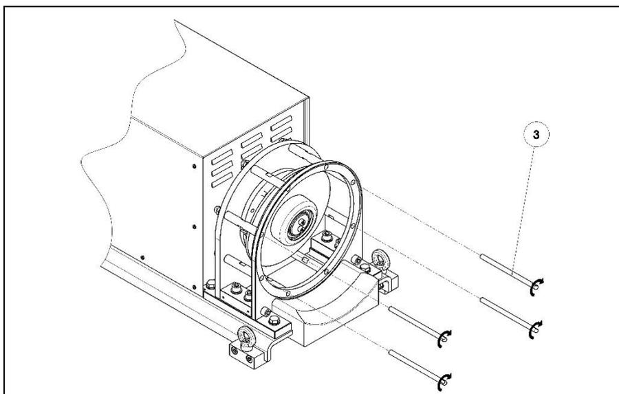
Screw in the track-units clockwise (item 3) into the thread holes of the ring-drive-unit.
