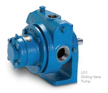
pumps have cavitation-suppression features that enable them to better handle any LPG vaporization that may occur within the pump. Finally, the LG1 pump incorporates a combined relief/bypass valve which limits discharge pressure. The combined valve also protects the pump from over-pressurization where both the downstream connection and the back to tank bypass connections are blocked.
