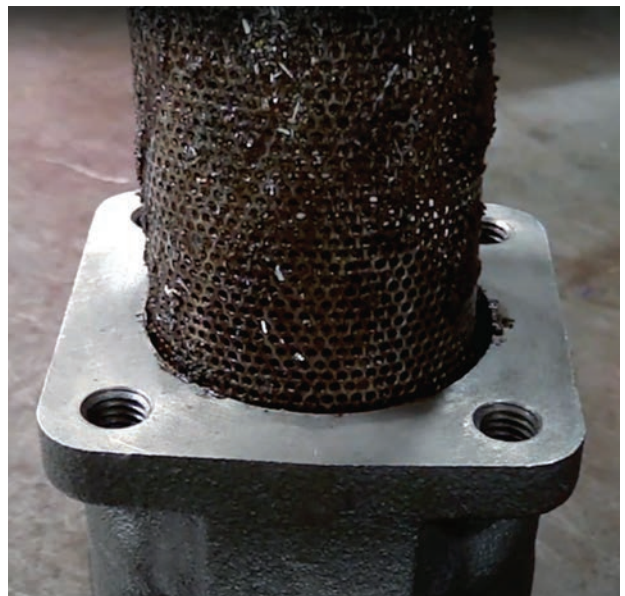
Clogged strainers signal suspended solids, which are a legitimate threat to most process pumps.
