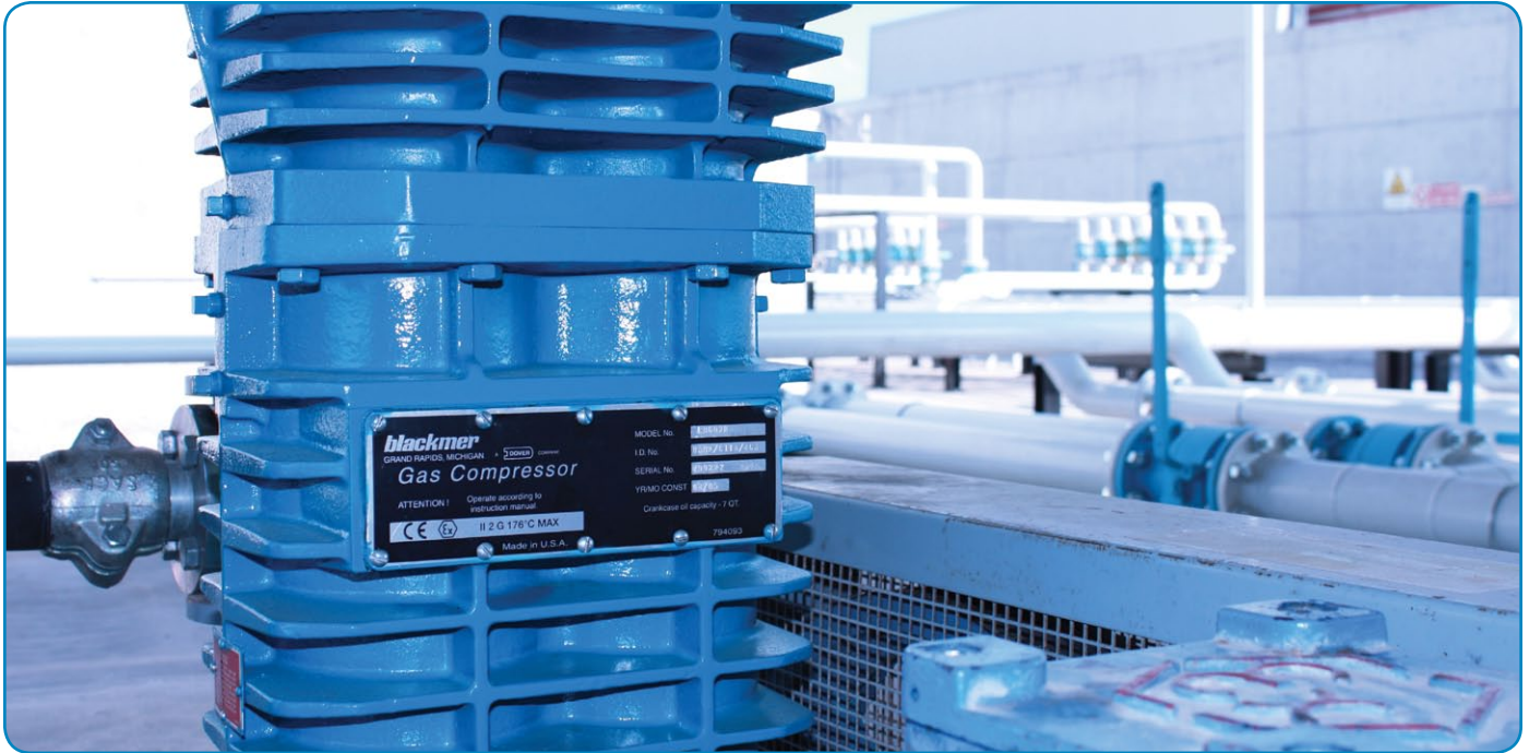
Blackmer's LB602 Single-Stage, Oil-Free Reciprocating Gas Compressor is one of the key pieces of equipment in use for LPG transfer and vapor recovery at the Maniago plant. The plant also uses Blackmer pumps.
