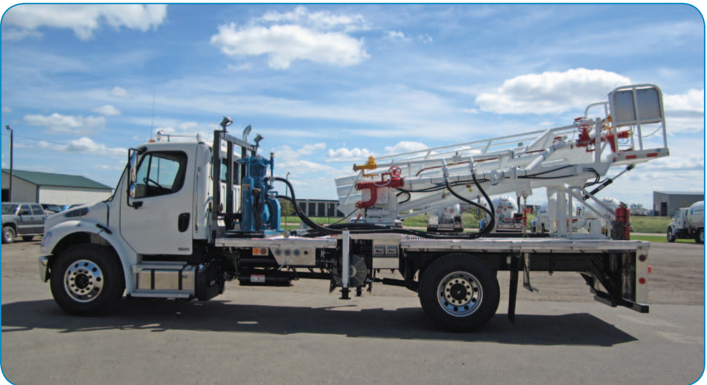
A Blackmer® LB601-LU Reciprocating Gas Compressor is mounted on the bed of the mobile LPG transloader and runs off the truck’s power takeoff (PTO) during product-transfer activities.
