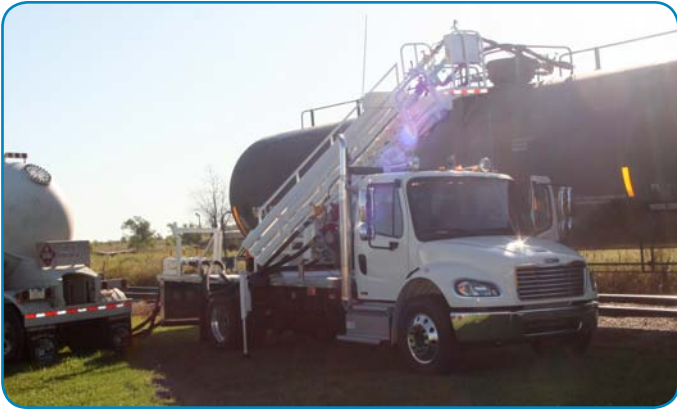
The CHS mobile transloader has traveled as far as Idaho to assist in a variety of LPG-offloading operations.
