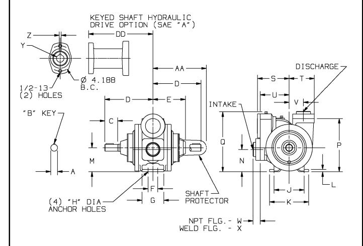
OPTIONAL PIPE CONNECTIONS: 2" NPT FLANGE, NODULAR 2" WELD FLANGE, STEEL
