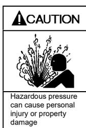
**Operating pump against a closed valve can cause system component failure, personal injury and property damage**
