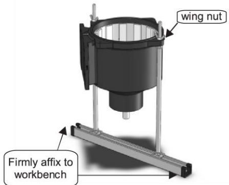
OUTER DRIVE ASSEMBLY MOUNTED TO TOOL
