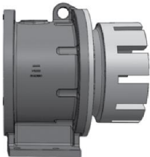
ROTOR INSTALLED INTO CANISTER
