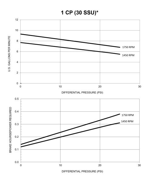
Blackmer Characteristic Curves are based on Brake Horsepower (BHp). To determine Motor Horsepower, drive train inefficiencies must be added to the BHp.
