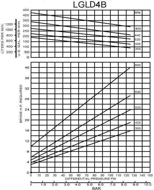
**NOTE:** Blackmer Characteristic Curves are based on Brake Horsepower (BHp). To determine Motor Horsepower, drive train inefficiencies must be added to the BHp.
