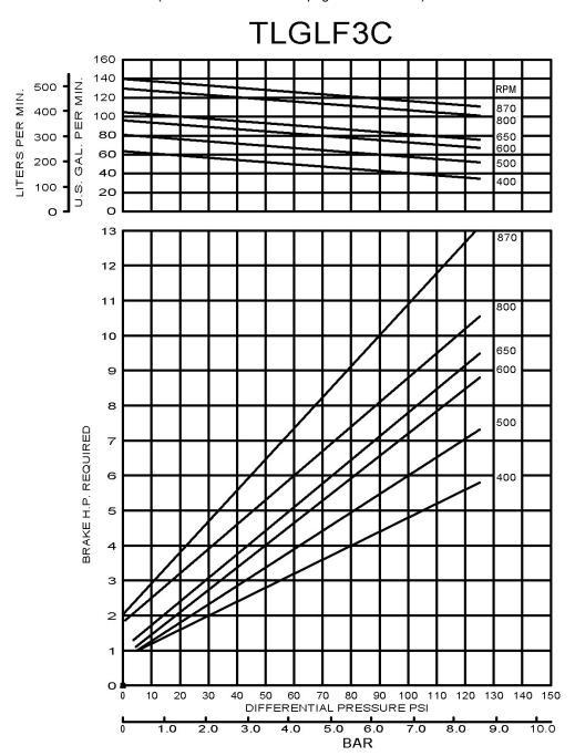
**NOTE:** Blackmer Characteristic Curves are based on Brake Horsepower (BHp). To determine Motor Horsepower, drive train inefficiencies must be added to the BHp.
