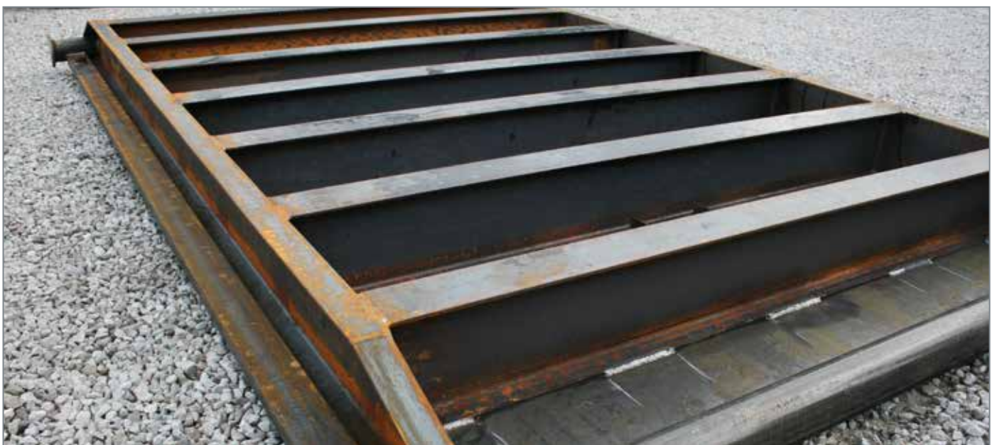
A key to effective vapor-recovery unit operation in the oilfield is the skid on which it rests. This skid assembly must be the proper weight and anchored correctly if it is to effectively absorb the the shaking forces and moments that are produced by the VRU's compressor.
