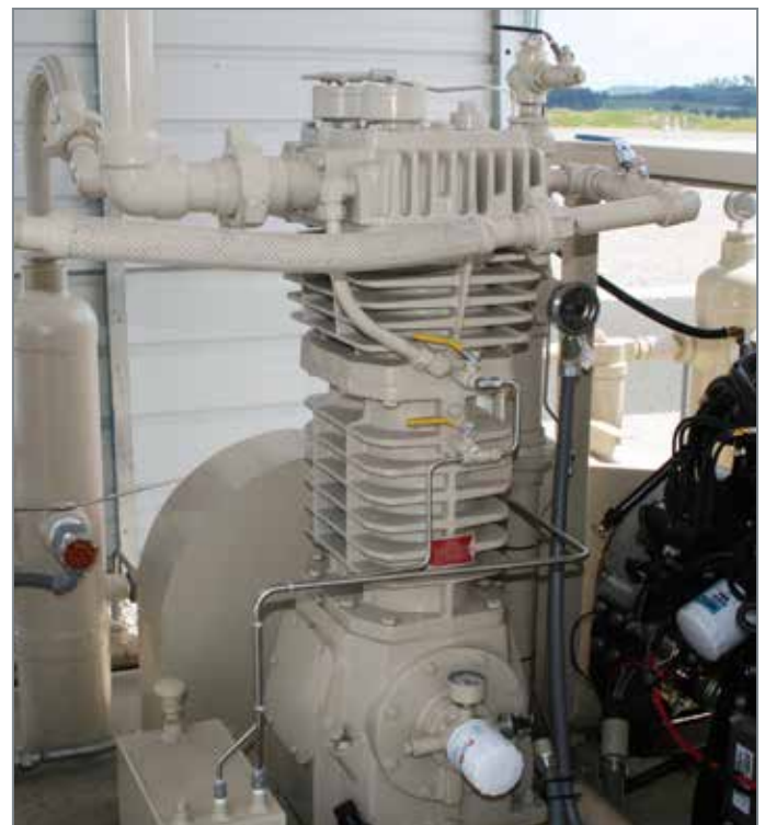
Blackmer® offers its HD (shown), HDS and NG Series models of Reciprocating Gas Compressors for use in oilfield applications.
