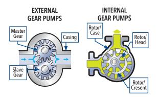
Gear pumps can be classified in to two main categories – internal or external. External gear pumps use two separate shafts to support two interlocking gears, which form a mesh at the center of the pump to move fluid along. Common gear types include helical, spur or herringbone gears to move liquid through the pump.
