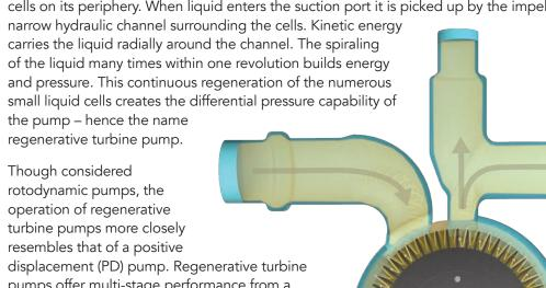
displacement (PD) pump. Regenerative turbine pumps offer multi-stage performance from a single-stage impeller that optimizes hydraulic performance, resulting in high differential pressures even at low flow rates. The pumps feature a compact design with few rotating and wearing components, which eases maintenance and repair demands.
