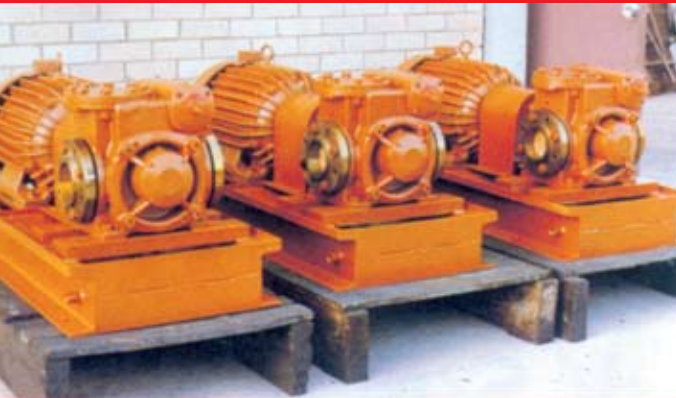
Electric Motor driven units
