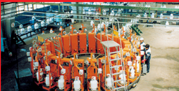
LPG carousel filling/bulk transfer
