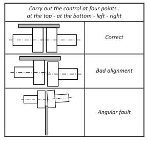
**REMINDER** : A flexible coupling does not avoid to do a good alignment.
