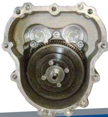
Torque limiter integrated into the PTO module
