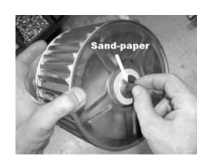
Mount without forcing the fan on the motor's shaft.
