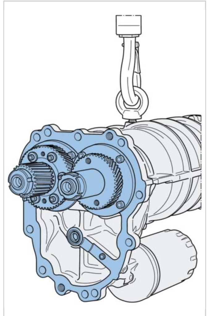
Remove plug of lubrication hole and lubricate lip seal **A**.
