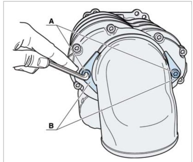
Remove the elbow **C** together with relevant O-ring.
