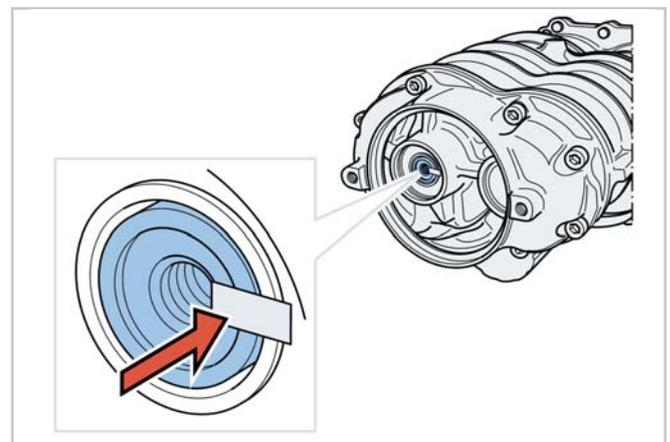
Fit the protection grid onto the suction port.
