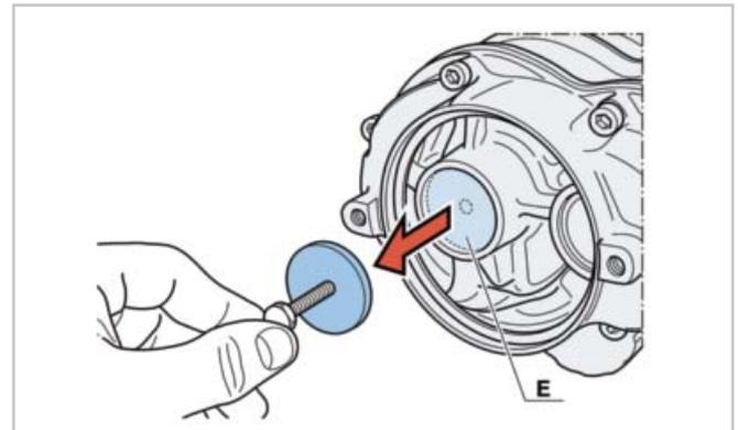
Stick a reflecting strip on the end of the screw shaft.
