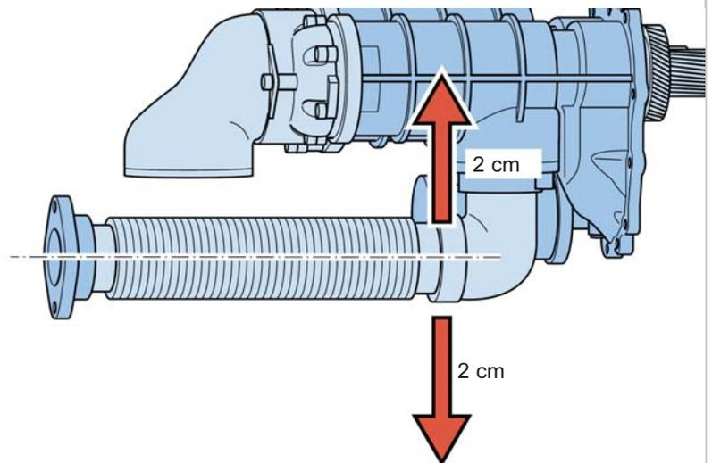
The angle of inclination of the flexible hose should be at most 45°.
