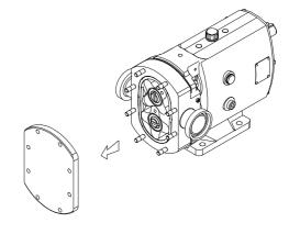
Step 2 Removing rotors
