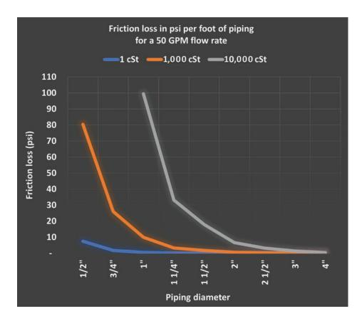
If we build the installation with 1.5" piping, the resulting differential pressure on the pump ports will be 133 psi. If the differential pressure is within the selected pump limits, the installation will operate without issues.
