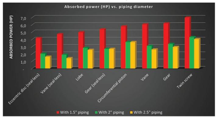
The appropriate approach is to check friction losses and differential pressure results with different pipe sizes and see which one offers the strongest energy consumption reduction. In the example above, 2" piping is the most balanced choice between piping enlargement and building cost.
