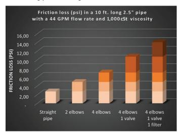
On this short section, depending on the design and ancillaries, resulting friction loss can be multiplied by five. Naturally, more pressure means more energy consumption.
