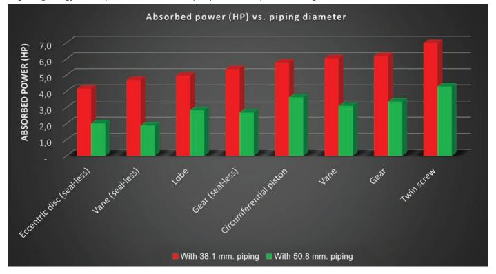
By selecting a slightly larger piping, power consumption and costs drop from 37% to more than 50%, depending on the selected pumping technology. By increasing the piping diameter and switching to a more energy-efficient pumping technology – like the Mouvex eccentric disc pump – the difference becomes exponentially greater, dividing the energy consumption by three in some cases.
