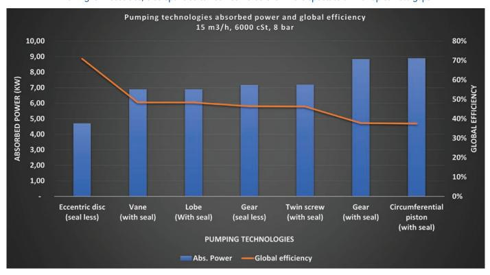
In both cases above and in most others, it is the same pumping technology that appears to be the most economical: The Mouvex® seal-less eccentric disc pump.
