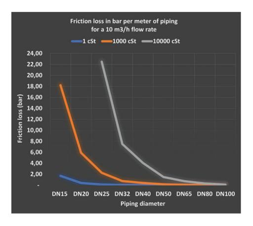
If we build the installation with 40 mm. piping, the resulting differential pressure on the pump ports will be 9.2 bar. If the differential pressure is within the selected pump limits, the installation will operate without issues.
