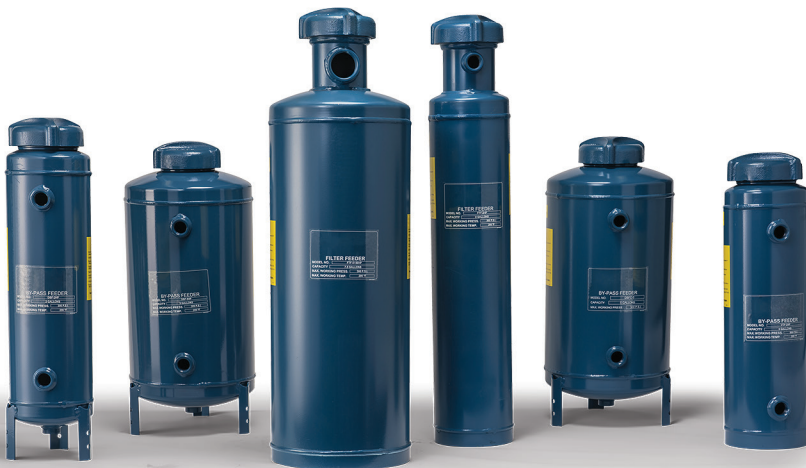
FIG. 3. Operating as a single piece of equipment that can inject water treatment chemicals while also acting as a filtration device, filter feeders continue to gain consideration for boiler water treatment because of this dual functionality.
