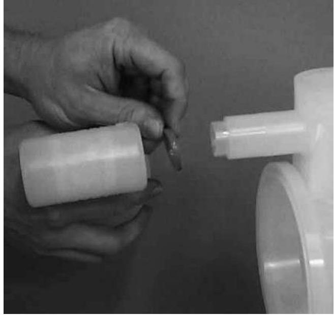
Step 11 Remove tee section from liquid chamber and inspect o-rings for signs of wear. Replace worn parts with genuine Wilden parts for reliable performance.
