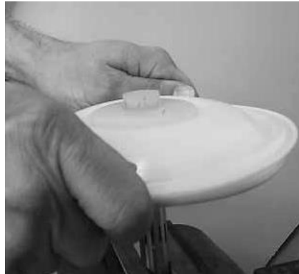
Step 13 To remove the remaining diaphragm assembly from the shaft, secure shaft with soft jaws (a vise fitted with plywood or other suitable material) to ensure shaft is not nicked, scratched, or gouged. Using hands or an adjustable wrench, remove diaphragm assembly from shaft. Inspect all parts for wear and replace with genuine Wilden parts if necessary.
