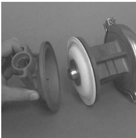
Step 10. Figure 10 Lift the liquid chamber away from the center section to expose the diaphragm and outer piston. (Figure 10)
