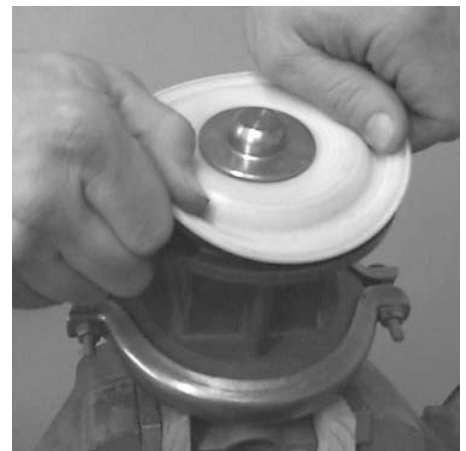
Step 11. Figure 11 Using an adjustable wrench, or by rotating the diaphragm by hand, remove the diaphragm assembly from the center section. (Figure 11)
